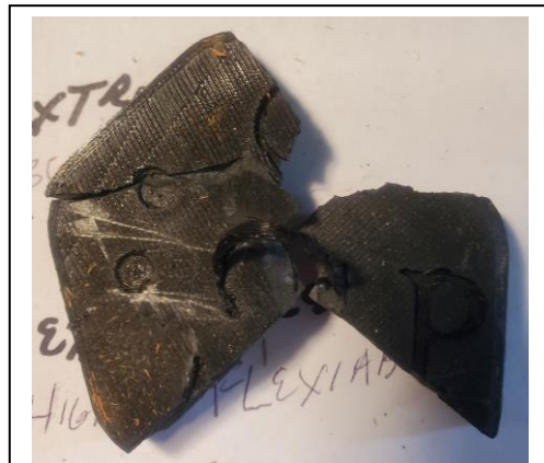
Shot test failure
