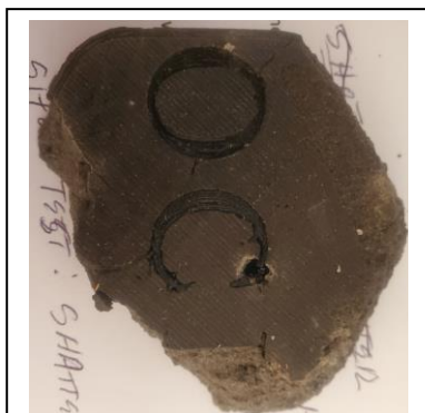
Shear strength test failure
