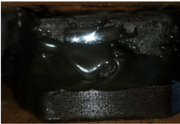
Stellamer-P tri-layer prepared for testing.
